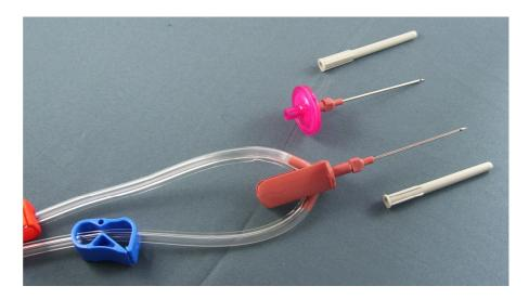
Pic. 1: Tubing with Needles and Vent Filter for SVP2
