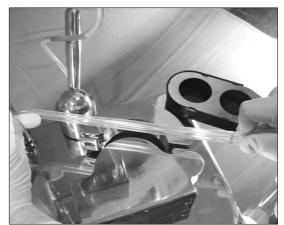
Pic. 4: Placement of PVC tubing in the Steripump head
