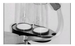
Pic. 3: Stericheck canisters placed on the drain tray
